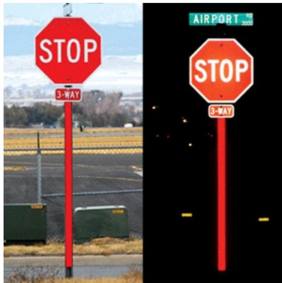
Figure 6. Retroreflectivity Visual Nighttime Inspection
