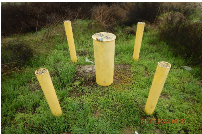
Photograph 5. Monitoring wells were locked.
