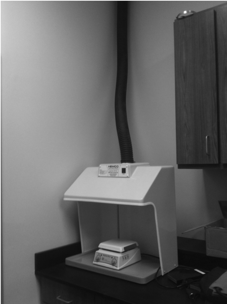
Figure 2: Benchtop fume hood installation
