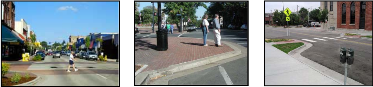
Figure 6.2. Examples of Pedestrian Bulbouts and Crosswalks
