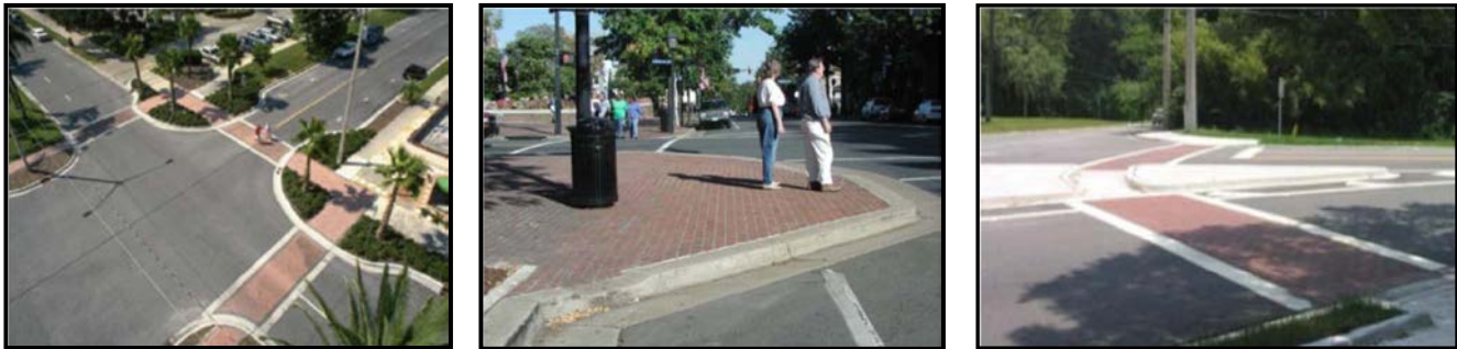
Figure 6.2. Examples of pedestrian bulbouts and crosswalks
